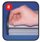
To open, **slide down both** locking tabs on the left and right sides of the base
