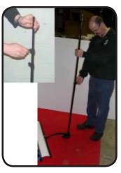
extend the middle section so telescopic pole only about 2.5" remain in the lower section.
