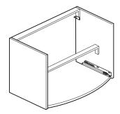
Place the unit centrally onto the lower bracket. Ensure it is level and mark all 4 fixing positions onto the wall. Remove the unit, drill Ø 6mm holes and insert the wall plugs.
