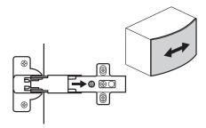
To move door left or right: Loosen screw shown and move door left or right to suit. Re-tighten.
