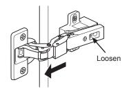
Remove the door before installation. Loosen the screw (shown) on both hinges, pull the door back and lift the hinges off the hinge plates. Remove the glass shelf.
