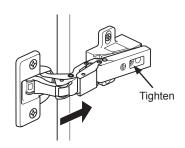
**Re-fit door:** Reposition both hinges over the screws on the hinge plates. Pull the door forward and tighten the screws. Re-fit the glass shelf.
