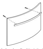
Attach door handle: Attach the handle to the door front. *Note:* Only attach the handle now if **not** changing the opening side (see below).
