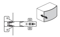
**To move door in or out:** Loosen screw shown and move door in or out to suit. Re-tighten.
