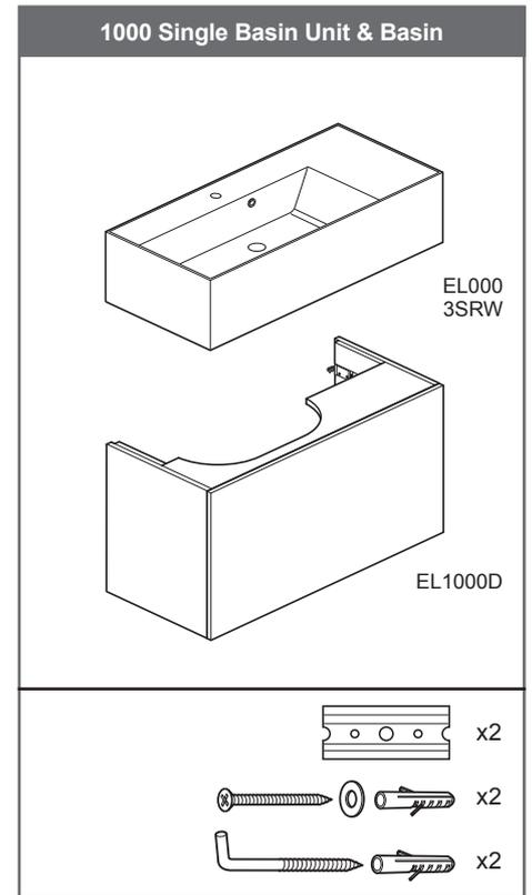
**Tools & equipment needed:** Drill, 8mm Suitable drill bit, Phillips screwdriver, Spirit level, Ruler/tape measure, Pencil, Silicone sealant (clear).
