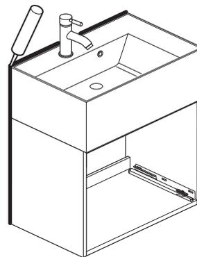
**a:** Attach the tap to basin and carefully bed in the waste using silicone **only**.
