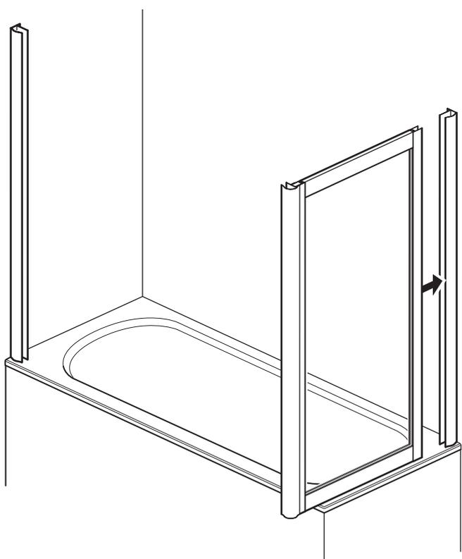
Insert the end panel into the wall channel and position correctly on the bath.
