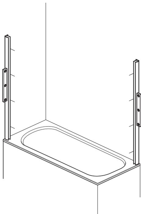
Remove both wall channels from the door frame. Place each wall channel in position on the bath (10 - 15mm in from the outer edges of the bath), use a spirit level to ensure they are vertical and mark all 8 fixing holes onto the walls (holes inside).
