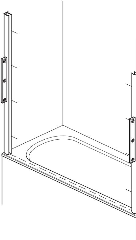
Remove both wall channels from the door frame. Place each wall channel in position on the bath (10 - 15mm in from the outer edge of the bath), use a spirit level to ensure they are vertical and mark all 8 fixing holes onto the walls (holes inside).
