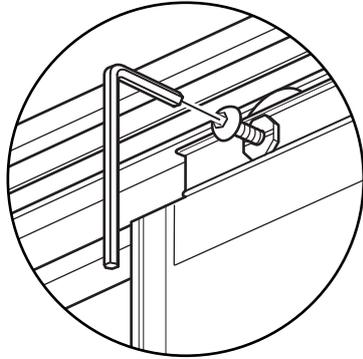
**If the door is not square with the fixed panel or doesn't close correctly, one or both of the top sliders should be adjusted.**
