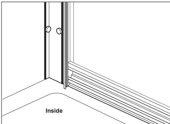
Before sealing you must make sure that the door opens and closes correctly.
