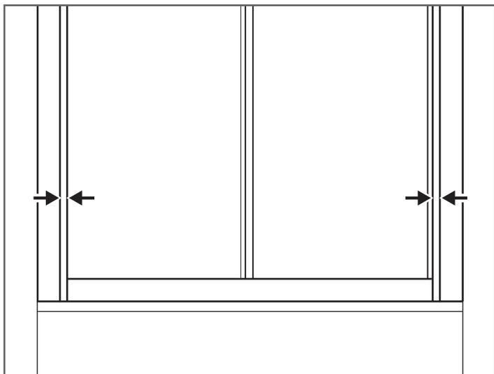
Before fixing the door to the wall channels you must make sure that the door is centred between the wall channels.
