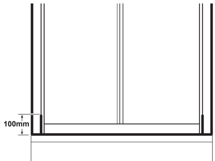
**Sealing outside:** Run a line of silicone sealant from top to bottom down the joint between the wall channels and tiles. Run a line of silicone sealant 100mm up the joint where the door slots into the wall channels. Run a line of sealant along the base in the joint between the bottom of the enclosure and the bath, from wall to wall.
