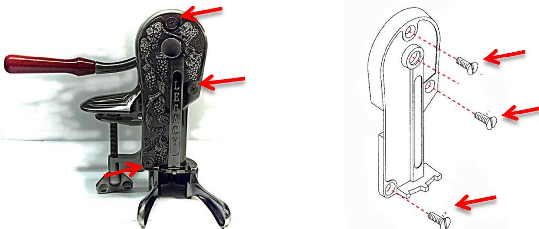
**Step #3. Replacing the Worm and Guide Slug.**
