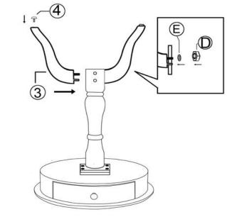
Insert legs into base holes as shown, and tighten nuts with washer up by wrench. And turn the adjustable hardware.
