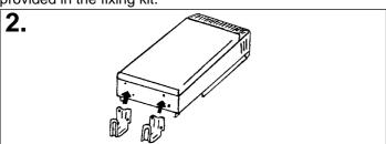
**3 XLS6N MODEL ONLY** - Attach the Room Sensor to the plastic clip which is located at the rear of the of the heater, as shown below.
