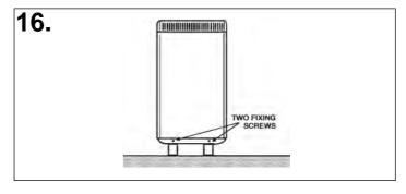
17. Check that the screws securing the heater to the wall bracket have been fully tightened.
