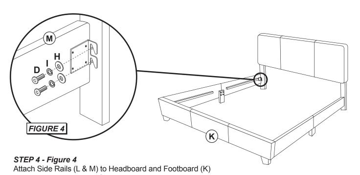
using 2 Allen Bolts (D), 2 Spring Washers (I) and 2 Flat Washers (H) per side. Tighten all bolts with Allen Wrench
