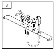
For models with spray (fits 4-hole sinks): Insert spray hose down through the support and sink. Attach the spray hose to the connection beneath the faucet by aligning the tabs on quick connector. Push quick connector housing firmly upward and snap onto receiving tube tab. Pull down moderately to ensure connection has been made.
