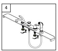
Insert spray hose through spray support and sink. Attach spray hose to spray hose nipple. Tighten with wrench.
