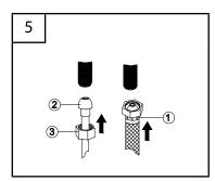
Make connections to water lines. Use 1/2" IPS faucet connections (1) or use the supplied coupling nuts (3) with 3/8" O.D. ball-nose risers (2) (not included). Use wrenches to tighten connections. Do not overtighten.
