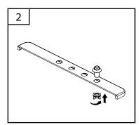
Insert sprayer support through far right hole on the sink. Screw the nut onto the shank from underneath the sink, hand tighten only.
