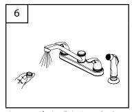
Important: After installation is completed, remove aerator. Turn on water supply and allow both hot and cold water to run for at least one minute each. While water is running, check for leaks. Replace aerator. Tighten nuts slightly to stop minor leaks. If problems persist, refer to troubleshooting chart.
