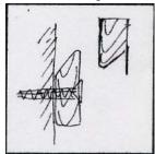
A hanger board may be fabricated using a 1x4, cut at a 45-degree angle. You may also cut a piece of wood that runs the length of the mantel shelf or use 2 blocks of wood that will be placed at either end of the mantel shelf. See above for measuring. Set the mantel on the length of wood or blocks. Use finishing nails on back side of legs (right underneath the back overhang of the shelf) to fasten to length of wood or blocks.
