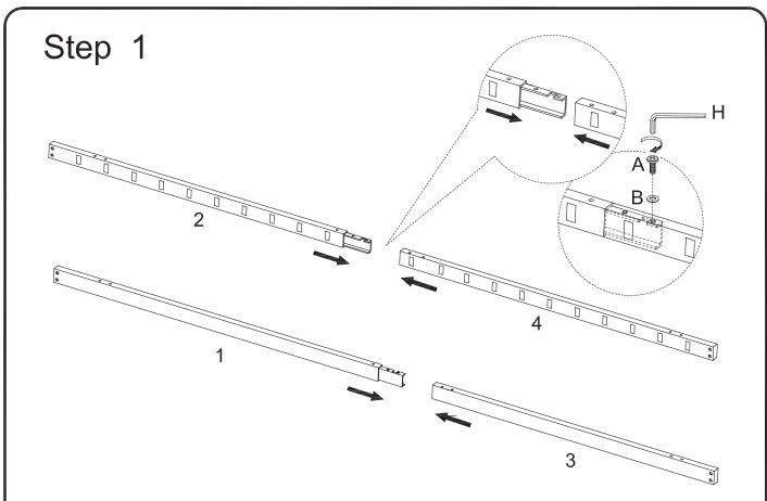
Slide rail (1) into rail (3), and rail (2) into rail (4). Secure rails (1,2) to rails (3,4) using small washer (B), small bolt (A) and small wrench (H).
