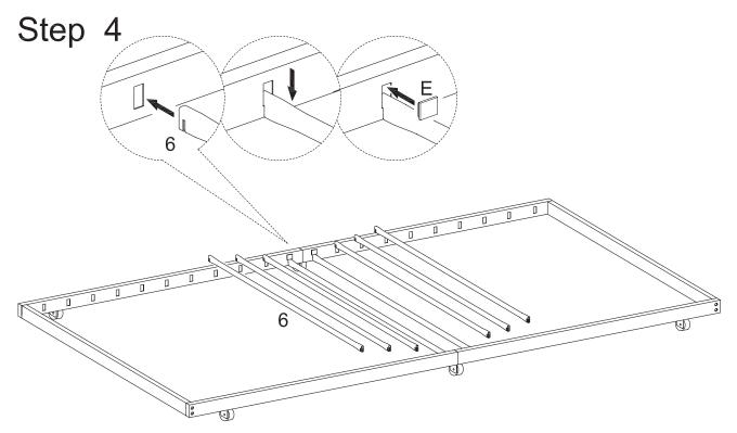
Carefully insert mattress support bars (6) into the slots of the rail assemblies from Step 1. Starting from the center and working out, secure mattress support bars (6) with plastic tab locks (E). First slide the left side of plastic tab lock (E) into the rail slot then snap the right side into the slot. It may be necessary to apply more pressure to some plastic tab locks than others in order to secure them.
