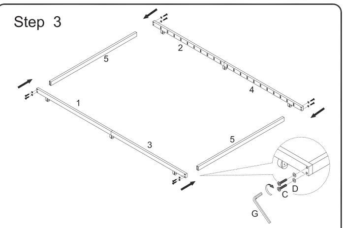
Attach rails (5) to the rail assemblies from Step 1 using large washers (D), large bolts (C) and large wrench (G).
