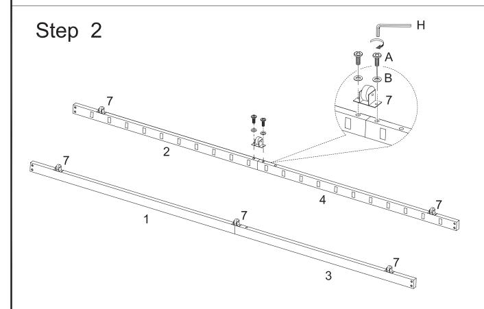
Attach wheels (7) to the rail assemblies from Step 1 using small washer (B), small bolts (A) and small wrench (H).
