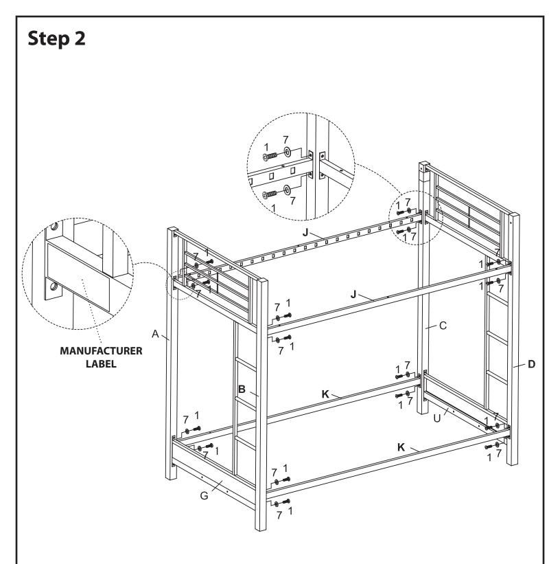
Join the end supports assembled in step 1 together using lower cross bars (K) and upper cross bars (J) as shown in the illustration.
