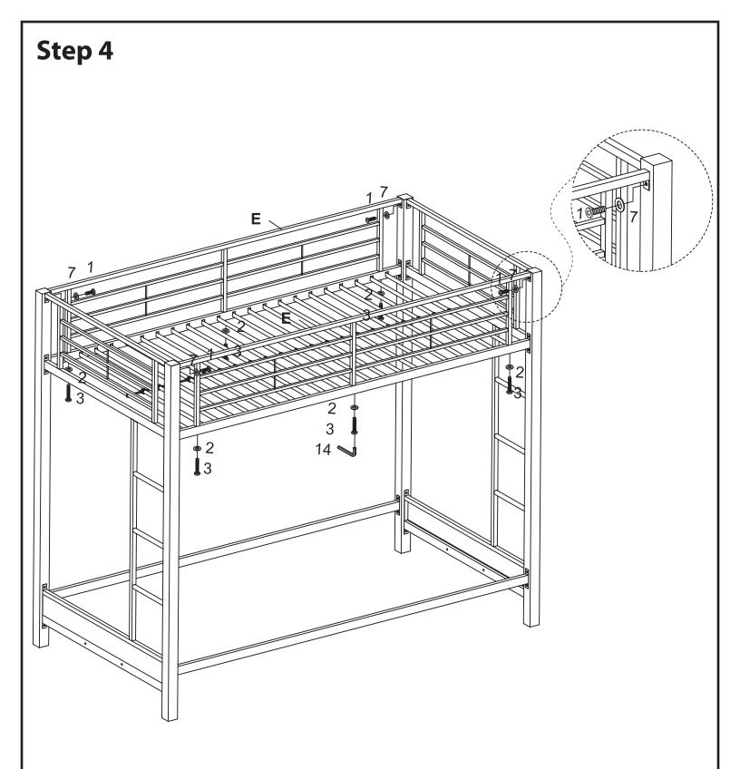
Attach upper guardrails (E) to frame support beams using screws (1) and washers (7) as shown in the illustration.
