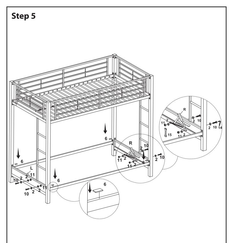
Attach adjustment mechanisms (L, R) to lower support using screws (10), washers (2), and nuts (11) as shown in the illustration. Tighten nuts using the provided wrench (15). Be sure to tighten all parts firmly.
