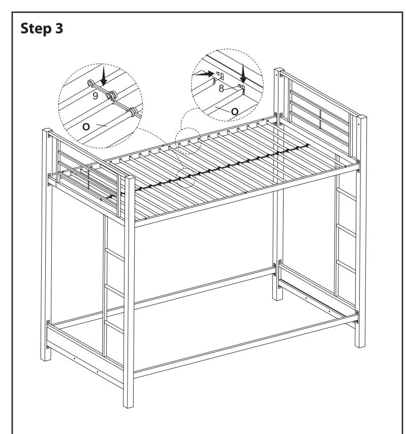
Insert upper mattress support bars (O) into the slots on cross bars (J) as shown in the illustration.
