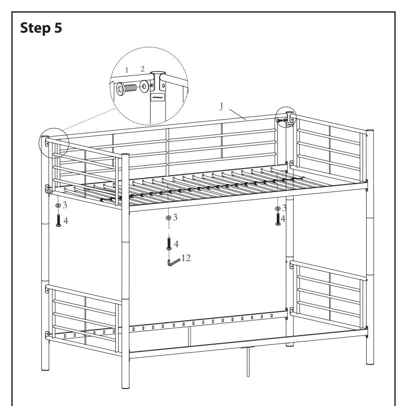
Attach back upper guardrail (J) to the back frame support beams using screws (1) and washers (2) as shown in the illustration.
