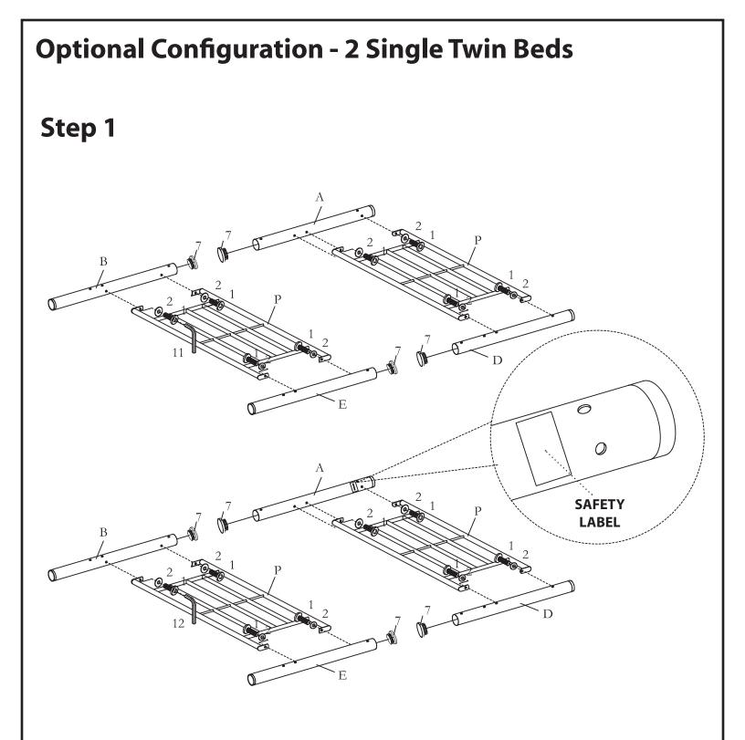
Attach end rails (P) to legs (A, D) and legs (B, E) using screws (1) and washers (2) as shown in the illustration. Attach plastic end caps (7) as shown in the illustration.
