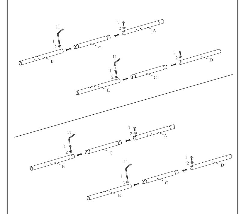
Assemble the four support posts by combining parts B, C, and A; then parts E, C, and D as shown in the illustration. Secure these parts together using screws (1) and washers (2).
