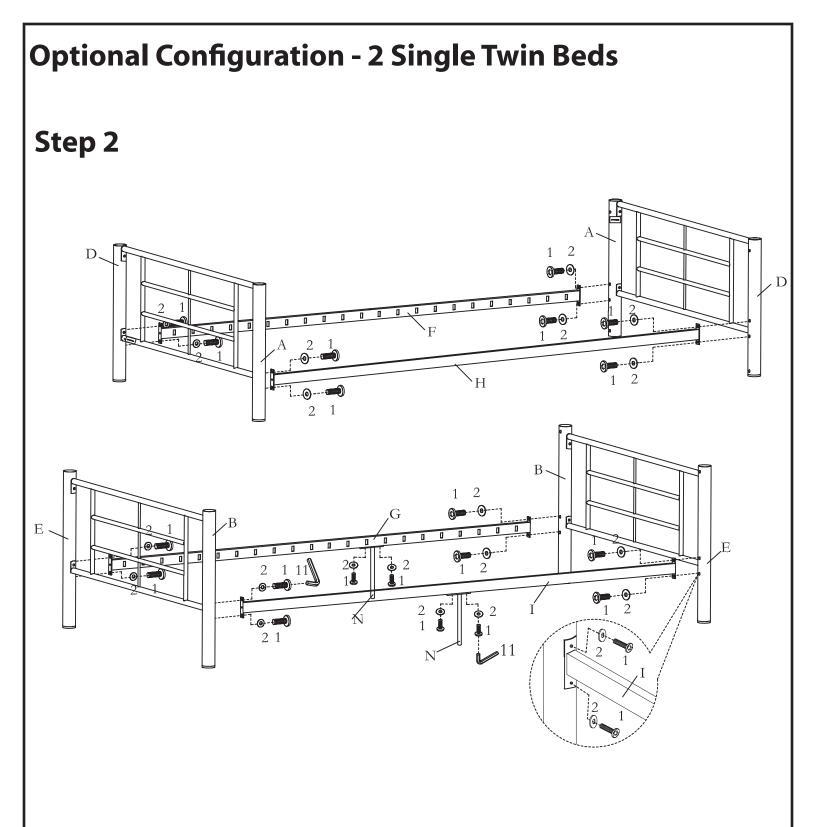
Join the support posts together using cross bars (F, H) and (G, I) as shown in the illustration.
