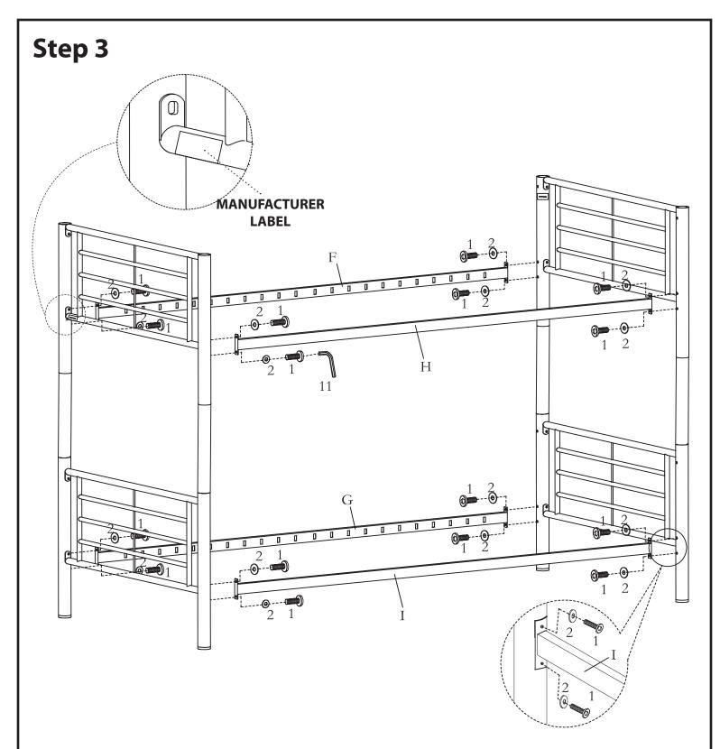
Join the end supports assembled in Step 2 together using lower cross bars (G and I) and upper cross bars (F and H) as shown in the illustration.
