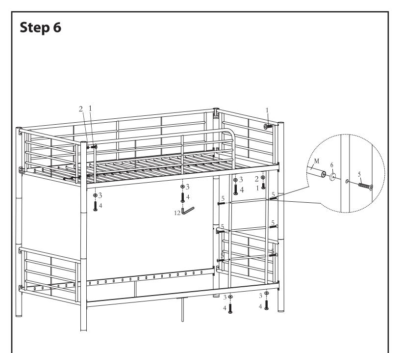
Attach ladder support posts (L) to the upper cross bar on the right side using screw (1) and washer (2) on the left side using screw (3) and washer (4) as shown in the illustration. Attach ladder support posts to the lower cross bar using screws (4) and washers (3) as shown in the illustration.
