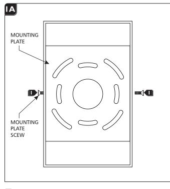
**I** Unscrew and remove the 2 mounting plate screws.
