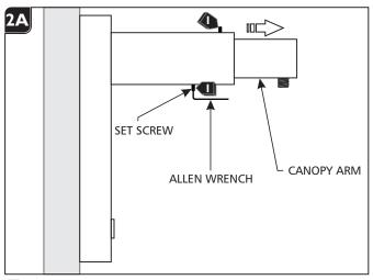
If needed, adjust the canopy arm's length by loosening the top and bottom set screws, pull the arm out to the desired position, and secure it in place by re tightening the set screws.
