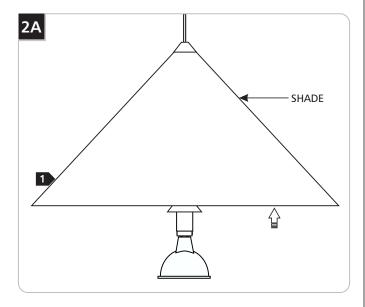
1 Slide the shade up on the wire to expose the socket.
