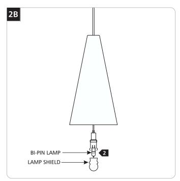
2 Remove the lamp shield and the old lamp.
