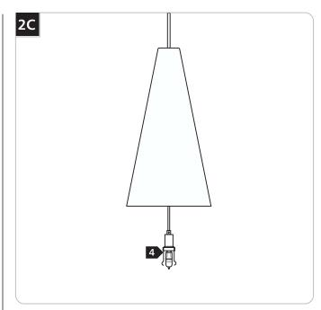
For incandescent versions, use MAX 50 Watt Bi-Pin Halogen Lamp.
