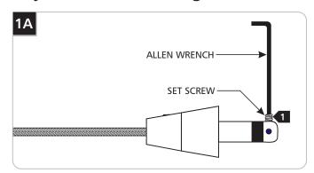
1 Back out (do not remove) the set screw on tip of the connector with the provided Allen wrench.
