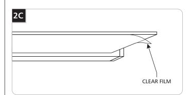
WARNING: DO NOT REMOVE THE WHITE ADHESIVE FILM from the top and sides of this fixture. Only REMOVE THE CLEAR PROTECTIVE FILM which is located on the bottom of the fixture.
