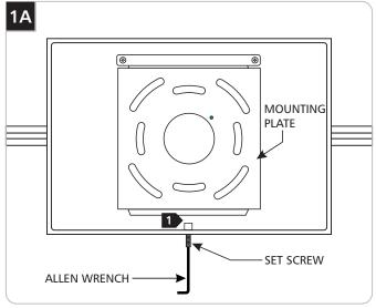
With the Allen wrench provided, back out (do not fully remove) the set screw at the base of the fixture.
