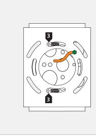
Attach the mounting plate to the electrical box using the two provided #8-32 screws .
