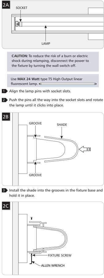
4 Secure the shade by installing the brackets and tightening the bracket screws with the provided Allen wrench.
