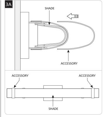
Slide the accessories onto the glass, until it snaps into place, at the desired location.
