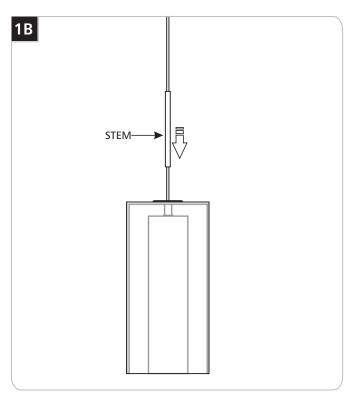
2 Install the stem onto the fixture cord and slide it completely down to the top of the outer shade.
