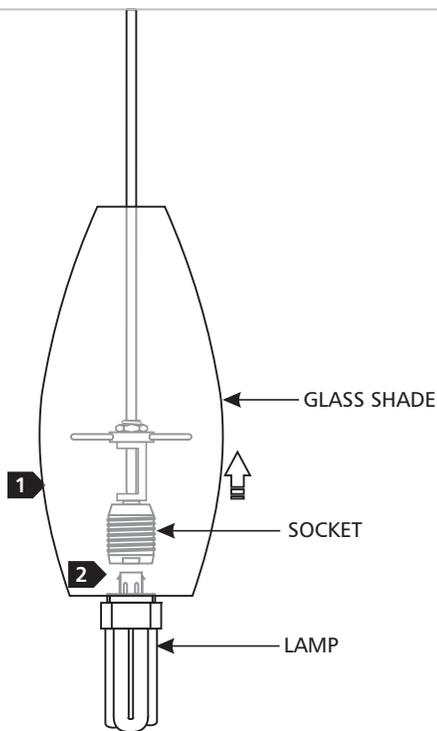
**CAUTION:** To reduce the risk of a burn or electric shock during relamping, disconnect the power to the fixture.
