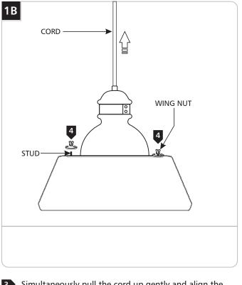
Simultaneously pull the cord up gently and align the studs with the holes on the glass shade.
