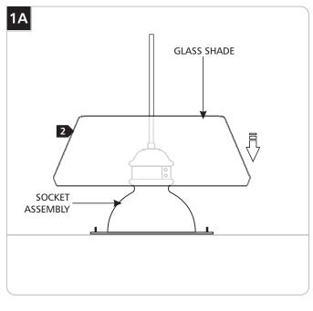
1 Place the socket assembly on a flat surface.
