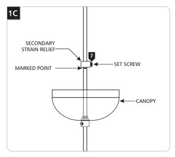
Feed the cord through the secondary strain relief. Place the secondary strain relief right above the marked point and tighten the set screw.
