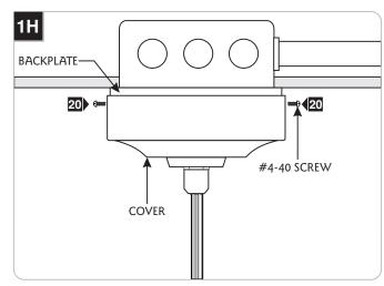
Line up the cover holes with the backplate holes. Replace and tighten the two #4-40 screws.
