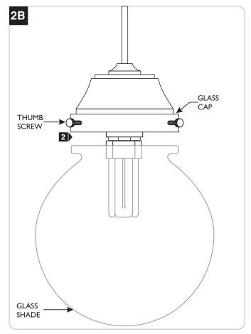
Place the glass shade completely into the glass cap and tighten the three thumb screws to secure the glass shade in place.
