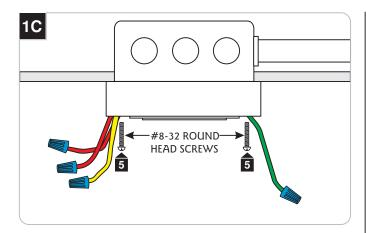
Place all power line wires and wire nut connections properly into the electrical box and mount backplate to the electrical box with the provided two #8-32 round head screws.
