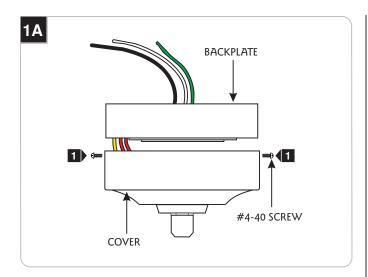
Remove the #4-40 screws on canopy sides to remove the cover from the backplate.
