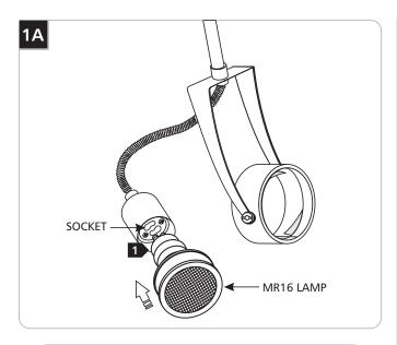
Use **ONLY 20 Watt** GX10 Base MR16 Ceramic Metal Halide lamp with models **700PJSSC162**\_.
