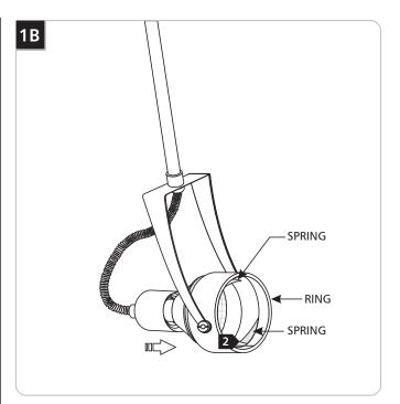
Push the lamp edge against the springs inside the ring until the edge of the lamp locks behind the springs.
