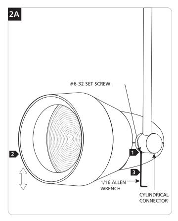
1 To lock the fixture head in a permanent vertical position, loosen (DO NOT REMOVE) the #6-32 set screw on cylindrical connector with the provided 1/16 Allen wrench.
