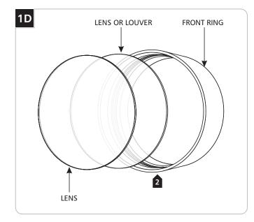
2 Place one or at most two lenses and/or louver into the front ring.
