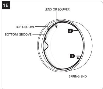
Squeeze the spring ends and place on top of the lenses (louver) and into the top groove of the front ring. Use the bottom groove if a single lens or louver is used.
