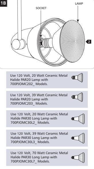
2 Screw the lamp into the socket.
