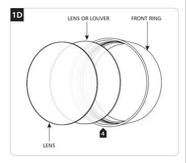
Place one or at most two lenses and/or louver into the front ring.
