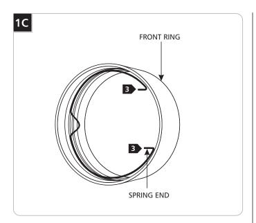
Squeeze the spring ends and remove it from the front ring.
