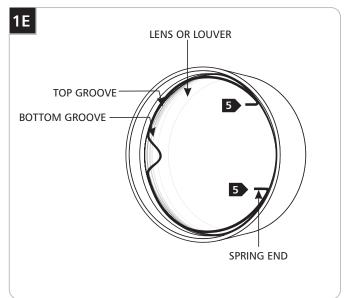
Squeeze the spring ends and place it on top of the lenses (louver) and into the top groove of the front ring. Use the bottom groove if a single lens or louver is used.
