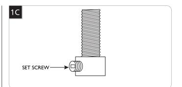
3 Loosen (Do Not Remove) the set screw on each strain relief.
