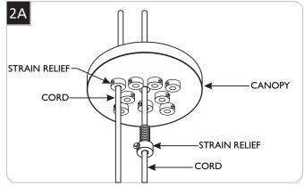
1 Feed a fixture cord through each the strain relief.
