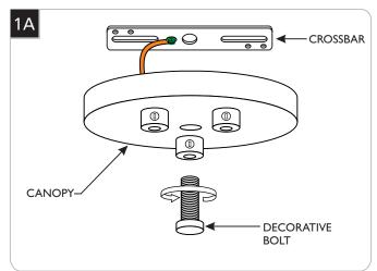
Remove the crossbar from the canopy by completely unscrewing the decorative bolt.
