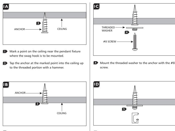
Screw the anchor in the rest of the way with a Phillips screwdriver.
