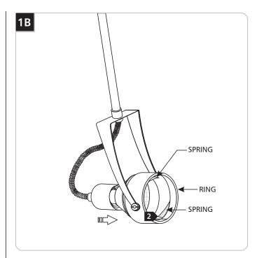
2 Push the lamp edge against the springs inside the ring until the edge of the lamp locks behind the springs.
