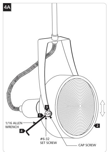
**1** To lock the fixture head in a permanent vertical position, loosen (DO NOT REMOVE) the #6-32 set screw on the edge of the cap screw with the provided 1/16 Allen wrench.
