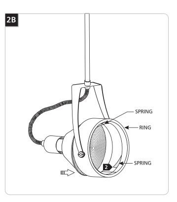
2 Push the lamp edge against the springs inside the ring until the edge of the lamp locks behind the springs.
