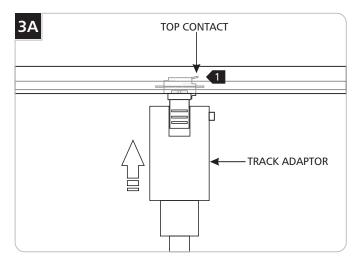
Push the Halo adapter contacts all the way into the Halo track.
