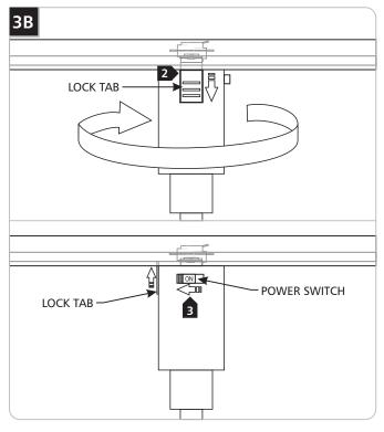
Pull down the lock tab, rotate the Halo adapter 90°, and release the lock tab.
