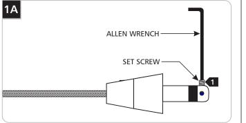
Back out (do not remove) the set screw on tip of the connector with the provided Allen wrench.
