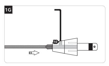
Tighten the #6-32 oval head set screw on the conical connector firmly.
