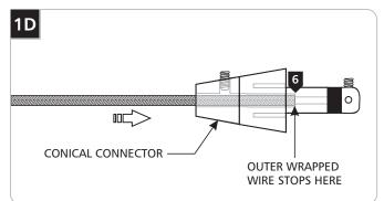
Feed and push the coaxial cable into the conical connector. The coaxial cable will come to a stop point after being inserted 3/4" into the conical connector.
