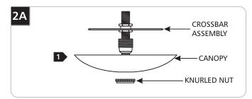
1 Loosen the knurled nut to remove the canopy from the crossbar assembly.
