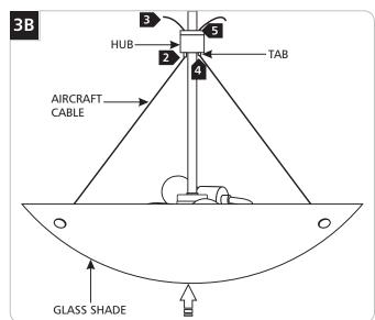
**NOTE:** Make sure to support the glass shade while adjusting the aircraft cables to position it in place as described in the steps below.
