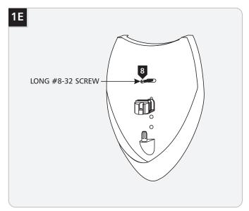
Align the top slot with the top inner threaded hole. Insert the long #8-32 screw through the slot and tighten it to the top inner threaded hole.
