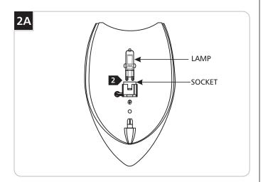
**NOTE:** The G9 lamp has an integral glass envelope and is thus safe to be used without a lamp shield.
