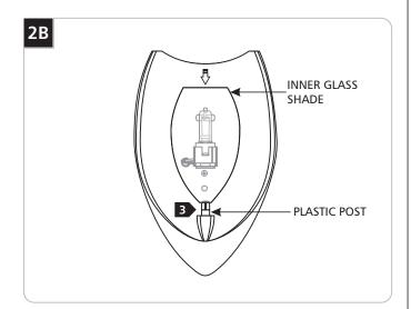
Align and push the inner glass shade completely onto the plastic post on the mounting plate and secure by sliding completely down.
