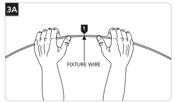
1 Bend the fixture wires to the desired shape by hands.
