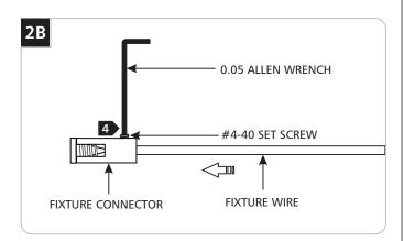
Feed the fixture wires into the fixture connector holes and tighten the #4-40 set screw with the 0.05 Allen wrench.
