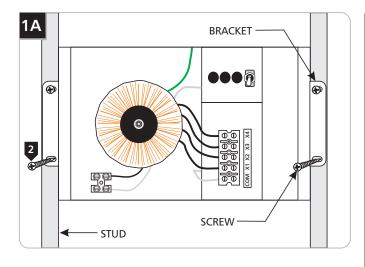
Select the location between the studs (16" apart) where the transformer is to be mounted.
