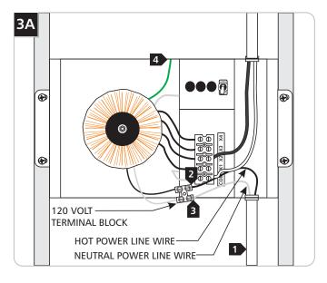
1 Install the 120 volt power line wires to the transformer.
