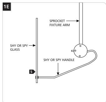
Rotate the Shy or Spy glass and the Sprocket fixture arm back to their original positions.
