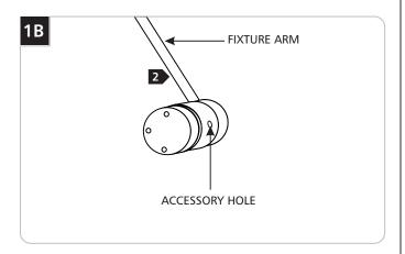
2 Rotate the Sprocket fixture arm away from the accessory hole.
