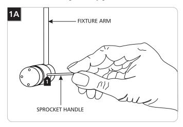
1 Unscrew the Sprocket handle. Use pliers if the handle is tight.
