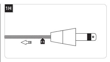
1 Pull the coaxial cable toward the fixture to smooth the wrinkles.
