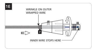
Keep pushing the coaxial cable into the connector while rotating the connector to ease feeding the inner wire into the tip of the connector. The outer wrapped wire will start wrinkling while being inserted another 1/2" into the connector.
