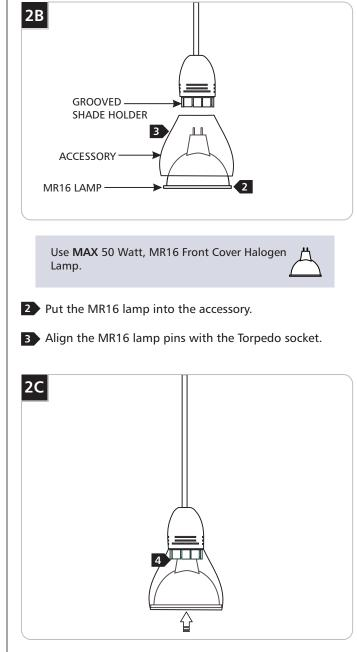
Push the lamp pins into the socket and simultaneously the accessory onto the grooved shade holder completely.
