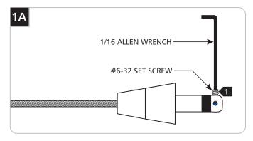
Back out (do not remove) the #6-32 set screw on tip of the connector with the provided 1/16 Allen wrench.
