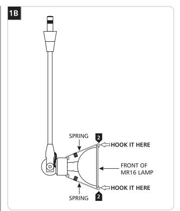
2 Gently pull the spring with thumb and forefinger, or a needle noise plier and hook the end onto front of the MR16 lamp so that it holds the MR16 lamp in position.
