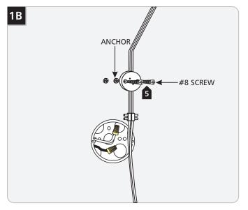
Mount the picture light bracket on the anchors with the two #8 screws.
