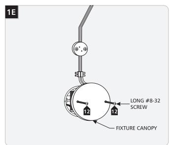
**NOTE:** Use the provided universal round crossbar when the canopy holes do not line up with the electrical box holes.
