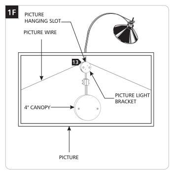
13 Hang the picture wire in the picture hanging slot on the picture light bracket.
