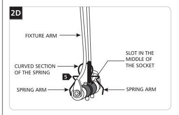
Snap the curved section of the spring onto the slot in the middle of the socket.
