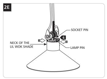
Squeeze the spring arms together and slide it into the neck of the Lil Wok shade while gently pressing the lamp pins all the way into the socket pins.
