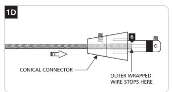
6 Feed and push the coaxial cable into the conical connector. The coaxial cable will come to a stop point after being inserted 3/4" into the conical connector.
