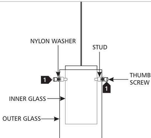
**1** Line up the outer glass holes with the inner glass studs and secure the outer glass to inner glass with provided thumb screws and nylon washers.
