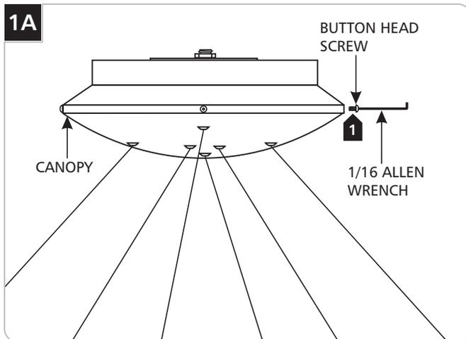
**1** Remove the four button head screws around the chandelier canopy with provided 1/16 Allen wrench.
