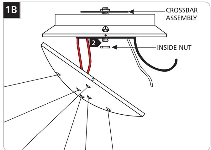
**2** Unscrew the inside nut to remove the crossbar assembly. *Do not disassemble the nipple from the crossbar.*
