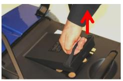
Once you swap the units. Make sure the battery is firmly locked in place. You will need to "Fully" charge the battery before operating the Mobie for the first time,
