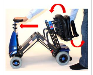
2. Carefully grab the control panel or tiller handle and push the Mobie forward while holding the seat.
