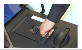
Swap the battery with the "dummy" battery cartridge as the label in the middle of the floorboard illustrates.
