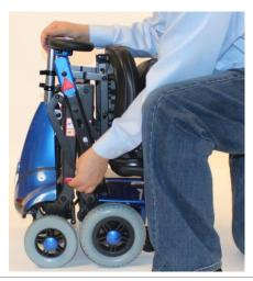
3. Grab the rear of the seat and pull it up while continuing to push the tiller forward.
