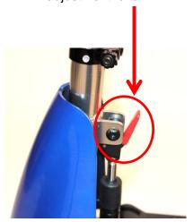
While you're holding down the lever, pull the tiller handlebar down until you find the proper adjustment to fit your body type.
