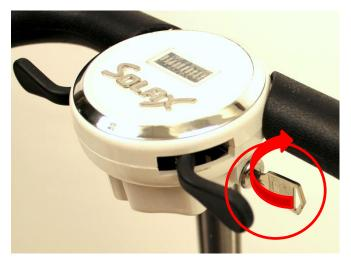
**Power On -** insert the key into the ignition and turn to the right.
