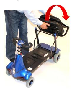
**6.** Grab the strap that is located in the middle of the floorboard and pull up while pushing the seat down.
