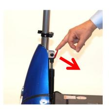
Follow the same procedure to readjust to the upright position. You will need to adjust to default position when folding the Mobie
