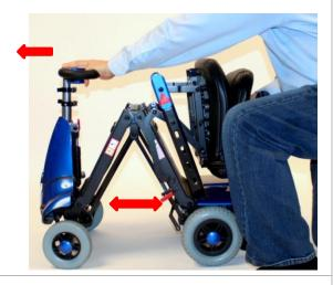
4. As the scooter unfolds, either push the floorboard down with your hand (avoid pinch point) or place your foot on the floorboard and press down until it locks in place. Do not place your foot in-between the "Pinch" point of your foot may get injured.
