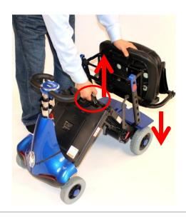
**7.** Push the front and rear chassis together until they lock in place.
