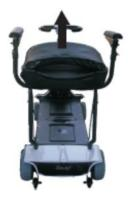
Lift the rear seat and lock into place
