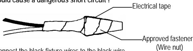
6. Connect the black fixture wires to the black wire in the outlet box. Fasten the joined wires as in step 5.
