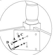
2. Attach all four legs to the desktop as shown in the circle diagram above. Place the lock washer (B) onto the allen screw first.Followed by the flat washer (C) and screw then into each leg.
