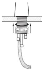
2. From under the sink, attach the plastic rings onto the faucet base, followed by the lock nut. Then tighten the two screws on the lock nut to secure the faucet body in place.
