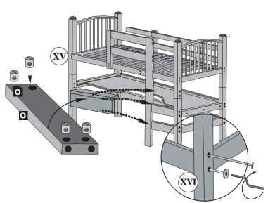
13) Locate the three ladder steps and position them on the loft as shown. Insert four barrel nuts for each step (See Diagram XV). Insert four 110mm bolts for each step (See Diagram XVI) tighten the bolts with the hex key provided.
