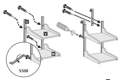
18) Insert four 50mm bolts through the two bookshelf upright supports unito the two shelves www. Notice that the larger bookshelf is located on the bottom. Tighten the bolts with the hex key provided (See Diagram XXIII). Attach two shelf brackets to the bookcase using four 5/8" inch screws. Use a phillips head screwdriver to tighten.
