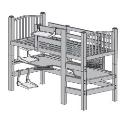
22) Congratulations, you are now ready to enjoy your loft bed. If you desire your loft to have left side ladder configuration, three things must be moved: The top headboards must be switched, the ladder assembly must be reversed, and the keyboard mounting bracket must be re-attached to the right side of the loft.
