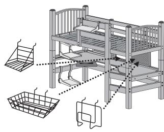
21) Locatethe three wire organizer baskets and attach them to the pegboard as desired. Attach the largest wire basket first and then the smaller ones. Attachment is done by tilting the basket (See Diagram XXIV) and inserting the prongs into the peg holes. Now push the basket back to a level position to secure the basket to the pegboard (See Diagram XXV).
