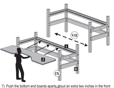
7) Push the bottom end boards aparts about an extra two inches in the front (Diagram VIII). Put the table top into the slot of the bottom end boards and slice the table edges back into the slot on the back rail (See Diagram IX). Note that the underside of the table has a pre-mounted left side keyboard bracket. The pre-drilled mounting holes are also on the right underside of the table should you wish to mount the keyboard on the right side of the table.
