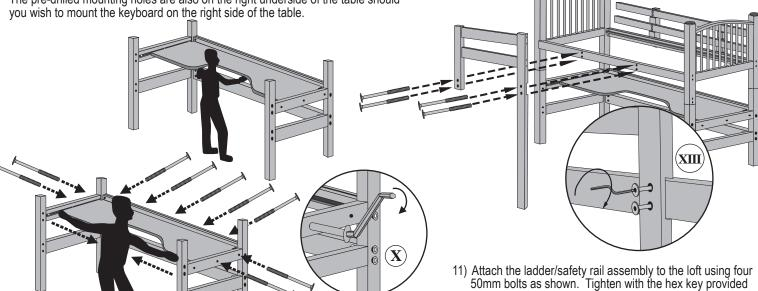
8) With the table top seated in the slots of the end boards, return the front legs of the end boards to their original position. Insert nine 2" JC screws through the end boards and upper slotted back rail into the edge of the desk and tighten with hex key (See Diagram X). Notice there will be one extra hole on each end board. Now fully tighten the eight 110mm bolts that attach the end boards to the back
