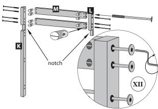
10) Locate the long upright support , the short upright support , and the two short front safety rails . Arrange as shown (See Diagram XIII). Be sure the notches of the long upright support and the short upright support are on the same side. Insert eight barrel nuts and eight 110mm bolts and tighten with hex key. (Reverse the layout if you desire a left hand side ladder).
