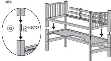
9) Insert four bunk connector oins into each of the corner posts of the lower unit, and place the loft bed assembly on top of the lower unit (See Diagram XI).
