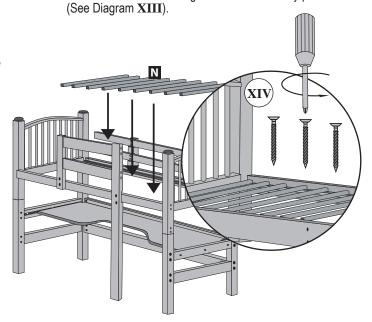
12) Unroll the slat bundle and lay it out on the loft as shown, strap side down. Attach slats to side rail ledge with slat screws using a phillips head screwdriver (See Diagram XIV). A power screwdriver comes in handy here.
