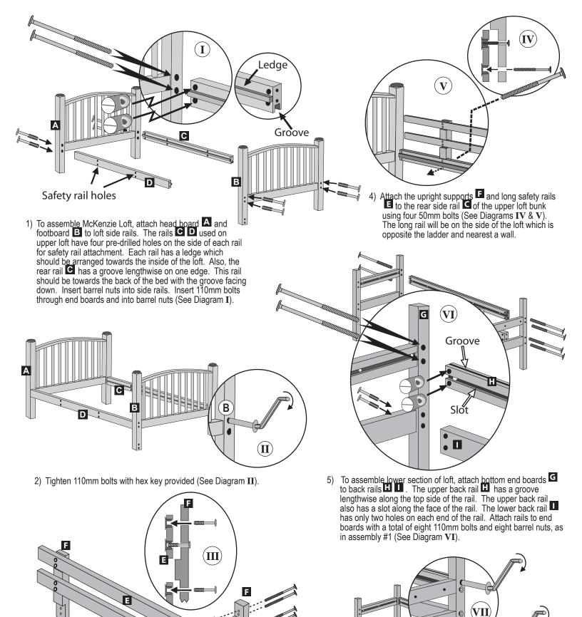
3) Attach the two long safety rails to the unassembled upright supports using eight 50mm bolts. Notice that the two long safety rails have sleeved, threaded inserts to connect the 50mm bolts. Tighten with hex key (See Diagrams III).
