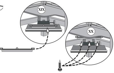
16) Loosen keyboard knob and slide the keyboard down and under the table. Now locate the plastic track guard and position it over the end of the keyboard track (See Diagram XIX). Use three 3/4" screws to secure the track guard over the edge of the track (See Diagram XX). Hand tighten with phillips head screwdriver. Do not over tighten as this may crack the plastic guard.
