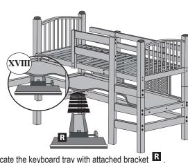
15) Locate the keyboard tray with attached bracket Slide the bracket into the track which is mounted on the underside of the desktop. (See Diagram XVIII).
