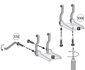
17) Attach the two printer/cpu brackets to the printer/cpu stand using the two 2" JC screws (See Diagram **XXI**). Tighten with allen wrench. Using a phillips head screwdriver attach two 5/8" screws to the bottom of each printer bracket as show (See Diagram **XXII**).
