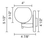
Suitable for dry locations only Mount to 3 1/2" - 4" round J-box Short circuit protection Overload protection Thermal protection
